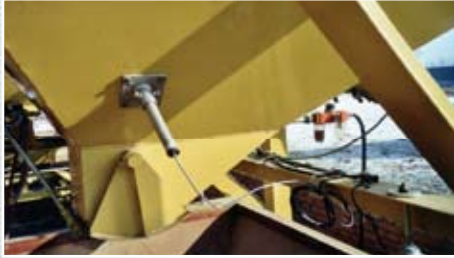
FSA - Arm mounted sensor with standard arm lengths of 0.2m, 0.5m or 1m. Appropriate for installation in silos (exterior view).
