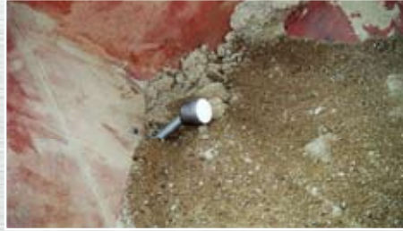
FSA - Sensor inside a sand silo. The probe is located directly inside the material flowing past the head. Negligible density variation during material flow.
